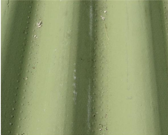
Photo 6. Non-ACM showing linear dimple pattern
