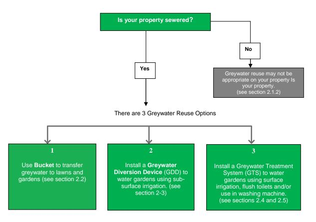
Each reuse option has different permitted end-uses and approval requirements. Tables 1 and 2 show how greywater can be reused depending on the treatment method and depending on whether it is for a single residence or a multi-dwelling/commercial premises
